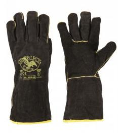
000507-0160 Cowhide split leather gloves, flame retardant treatment, 35 cm, fabric lining - Features: soft, strong, resistant - Strengths: comfort, easy to use, grip, protection, precision - Areas of application: precision welding and heavy-duty handling with hot, deburred material
